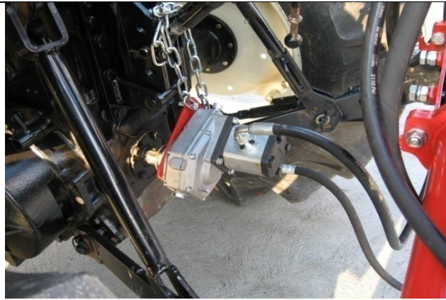
Figure 2. Hydraulic pump connected to the output shaft of the tractor
